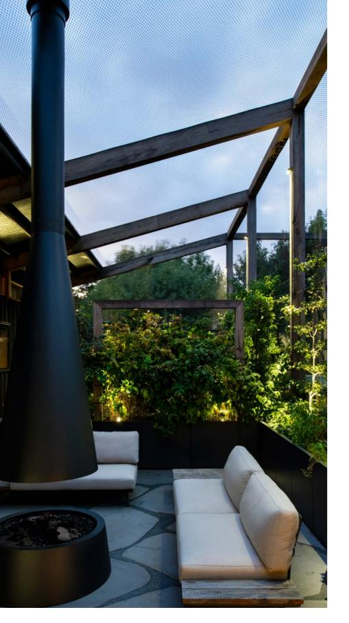
Nano floodlight proved to be the ideal lighting for the individual trees and the architectural structure. The floodlights with 38° beam were installed to light the foliage from the ground up, while Nano floodlight with a 14° beam was chosen to light up the wooden beams of the pergola.
